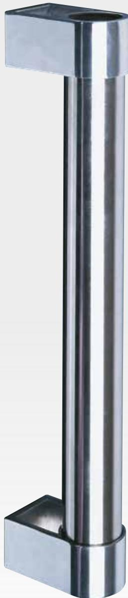
The Functional 97 series pull handles are manufactured using 41 mm diameter Satin Anodised Aluminium (SAA) tubing, or 38 mm diameter Stainless Steel, offered in Satin (SSS) and Polished (PSS) finishes.
