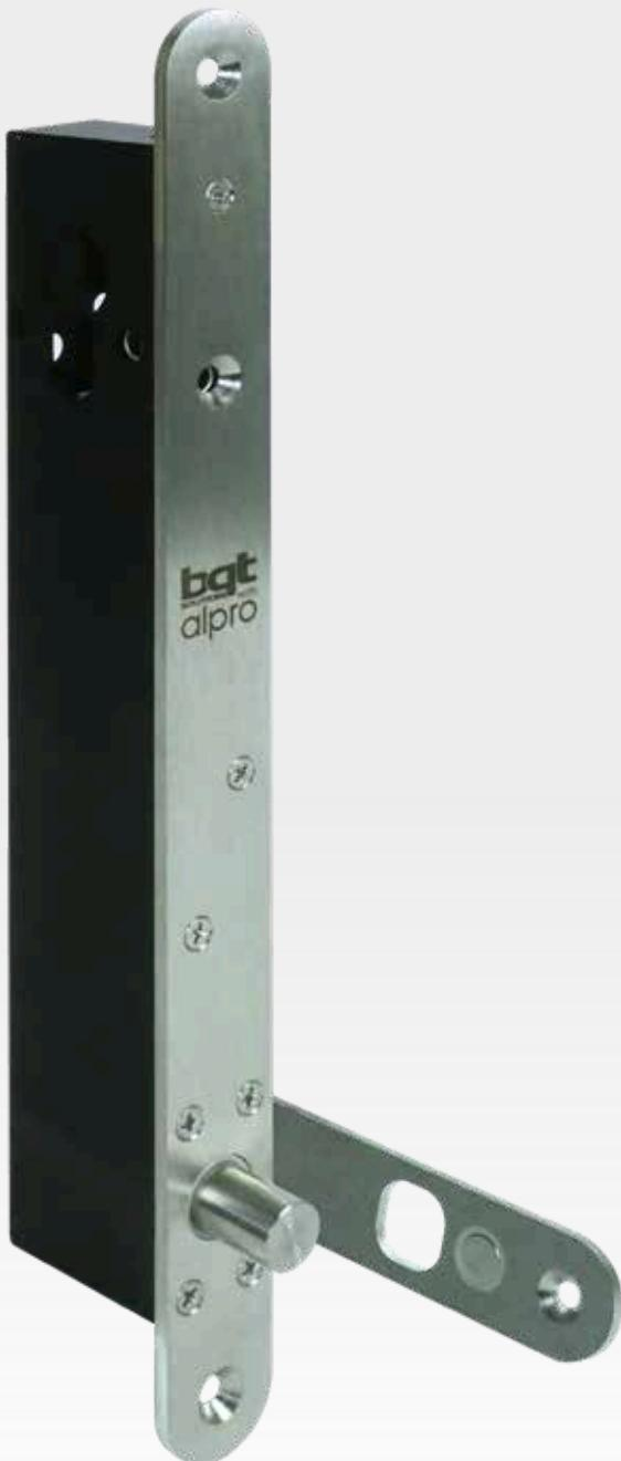
The Alpro DB25KO (key override) model offers the same functionality as the standard DB25 with provision for a Europrofile cylinder as a means of mechanical override. The ultra-slim design of the DB25KO enables fixing into very narrow sections. An advanced microprocessor module provides power reduction allowing continuous operation without heat generation as well as automatic voltage regulation.
