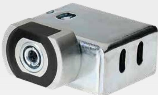
Alpro's patented AL4400 mechanical electro magnet is specifically designed for securing sliding door mechanisms, both automatic and mechanical. The holding force of the magnet will depend on its fitting arrangement, but in test the average holding force has been shown to be 680Kgs. The installation is simple and the unit provides an additional and reliable locking solution which is superior to traditional electromechanical locking devices.
