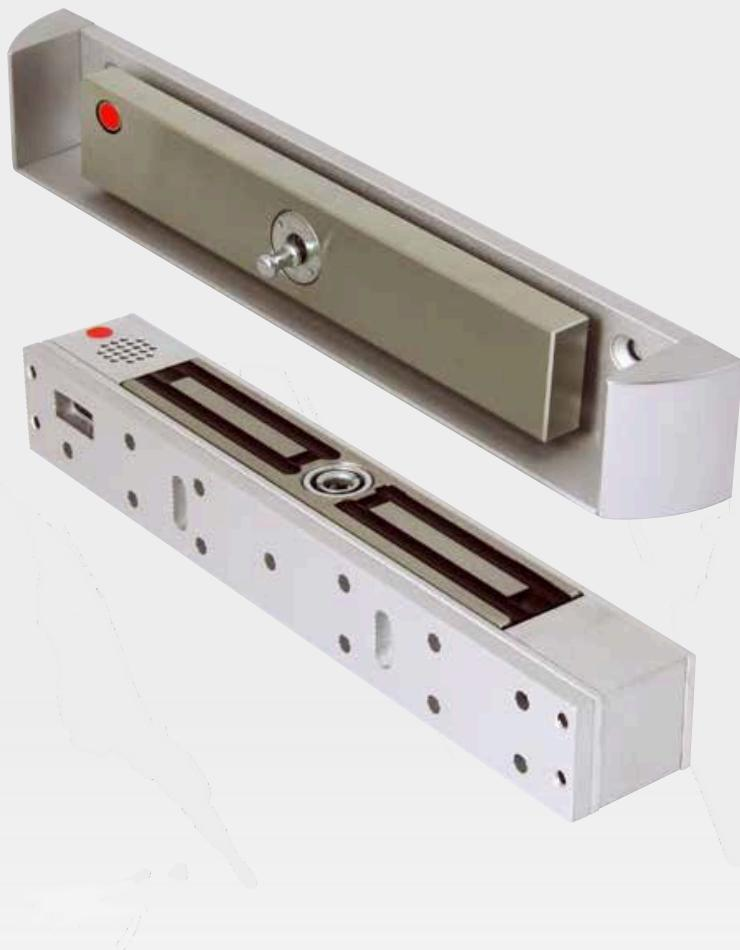
Alpro's Vortex 2400 compact door magnet is a unique magnet with patented inbuilt technology ensuring improved performance and reliability and a real alternative to standard face to face magnets. Complete with a conical aperture to receive a strong alloy pin the unit embodies both magnetic and mechanical holding force. Independently tested to 1500kg. Complete with built in LED and dual monitoring.
