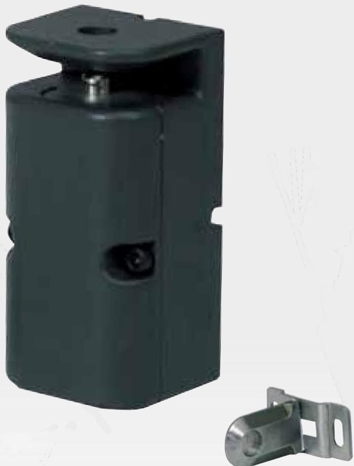
This compact rugged cabinet lock is designed to be fitted in display cases, cabinets and lockers with either swing or sliding doors requiring electronic control and where keys are not a practicable solution. The innovative design enables the lock to be fitted vertically or horizontally whilst receiving the striker plate from the front, side or slide entry positions. Offering maximum flexibility and alignment adjustment whilst maintaining an excellent level of security for its size.
