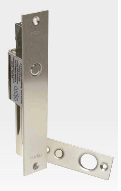
The Alpro EB1001 electric bolt allows for remote access and exit control of most timber and metal doors. It is suitable in sliding or swing, single and double action operations. It can be fitted in the frame or in the door and comes with plug in LED bolt indicator as standard.
