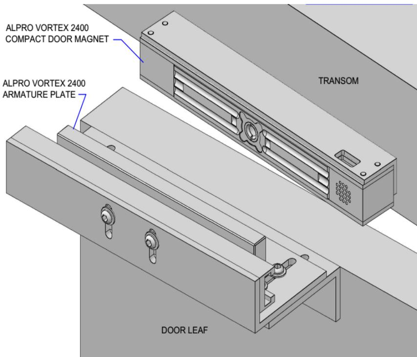
Installed magnet and bracket
